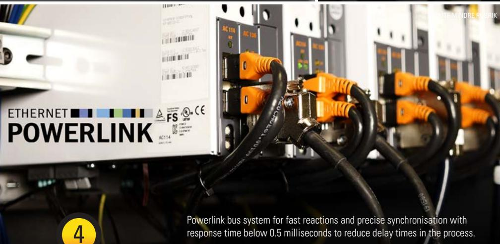
Powerlink bus system for fast reactions and precise synchronisation with response time below 0.5 milliseconds to reduce delay times in the process.
