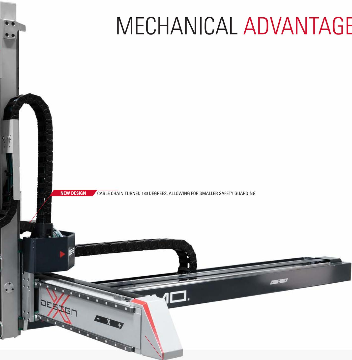
**NEW DESIGN** CABLE CHAIN TURNED 180 DEGREES, ALLOWING FOR SMALLER SAFETY GUARDING
